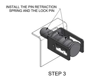
COMPRESS THE LOCK PIN AND RETRACTION SPRING.
