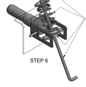
ASSEMBLE SPECIAL WASHER AND PIN ENGAGEMENT SPRING ONTO LINKAGE ROD AND GUIDE THROUGH THE SPRING CAGE PLATE.
