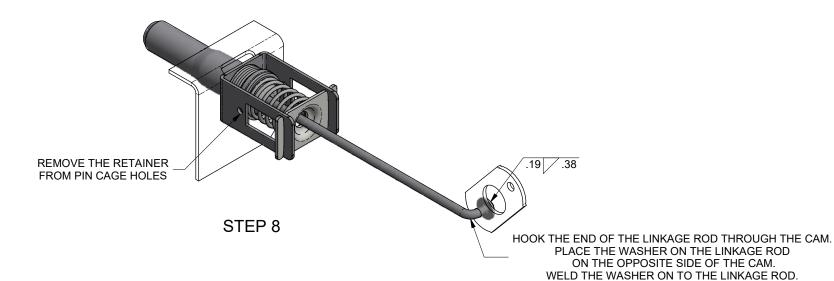
3. MAKE SURE LOCK PINS EXTEND AND FULLY RETRACT BEFORE PLACING SLIDER IN SERVICE.
