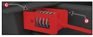
Not only does EZ-Pull 2 eliminate most of the problems associated with bound lock pins, it also reduces the effort needed to pull the pin release handle — a real work-saver!
