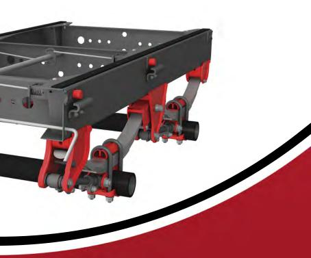
Corrosion-resistant individual hanger towers provide vertical load support.
